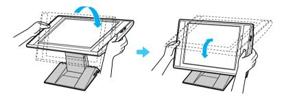
Set the display height so that it does not touch the keyboard, and adjust the viewing angle approximately 27 degrees from eye level to the center of the screen.
